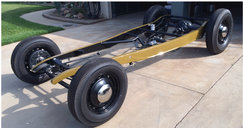
Like many car projects being finished in time for summer's sunshine, this modified "deuce" chassis is nearly ready for its vintage Chevy powerplant, Ford Model A body, Dodge truck grille and the rest of its parts.
