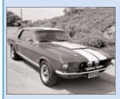
Specs (2001 restoration): Ford 302 motor, AOD transmission, Paxton supercharger, MSD ignition, disc brakes, eclipse sound system, and fiberglass front end from '67 Shelby.
